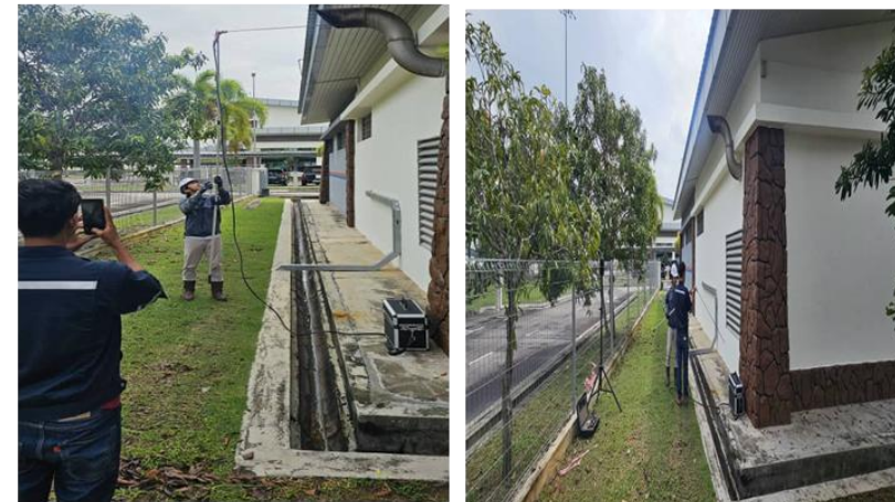
Smoke And Noise Test For Genset at LKSA
